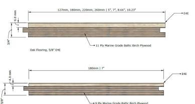
Quercus Robar is sourced from managed forests by our FSC certified mill in Europe. Logs are French Cut and the lamellas are graded to our custom specification. The sawn lamellas are bonded to an exterior grade baltic birch substrate, precision milled, filled as necessary, and sanded smooth.
